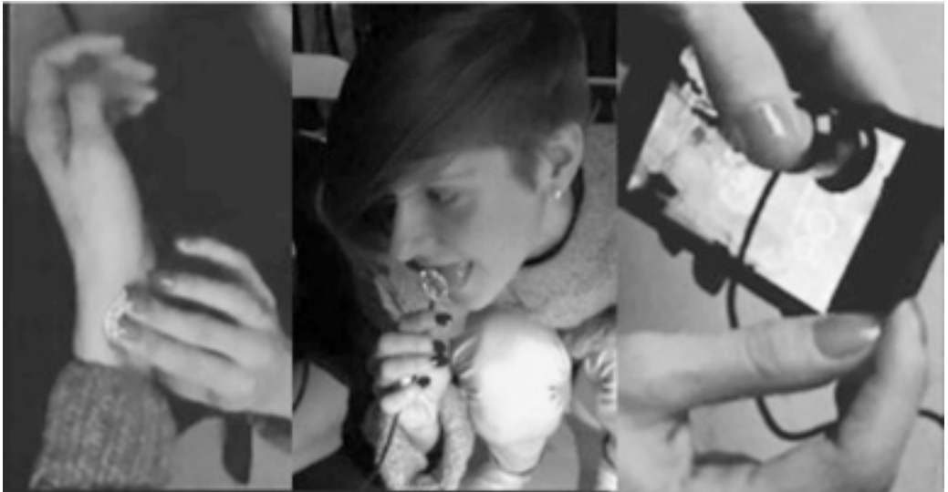
Figure 1. Contact microphones used to amplify the sound of participant's bodies and coil microphones used to amplify the processing sounds of smartphones.
