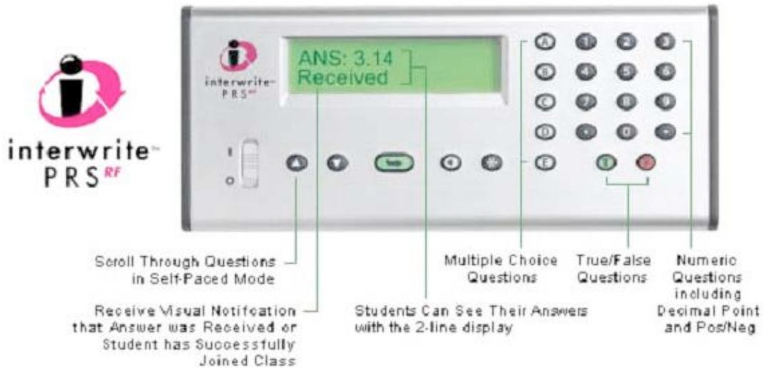
**Figure 2:** The "clicker", part of the PRS system from Interwrite [9] used in the study.
