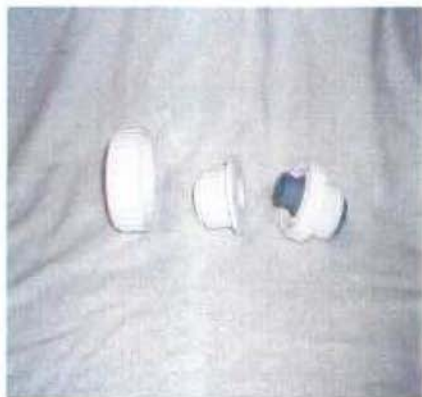
Fig. 1. Pieces of the eye model vessel: PVC union set and plumbing tubing.
