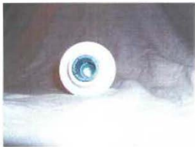
Fig. 2. Slits are cut into the larger diameter end (0.75 inch) of the plumbing tube for easier insertion of the porcine eye
